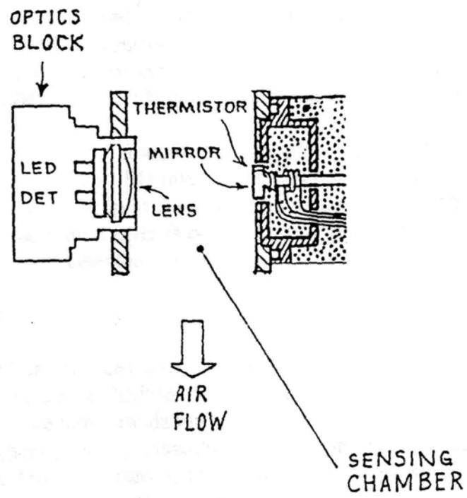
Fig. 4. Sensor assembly block diagram
