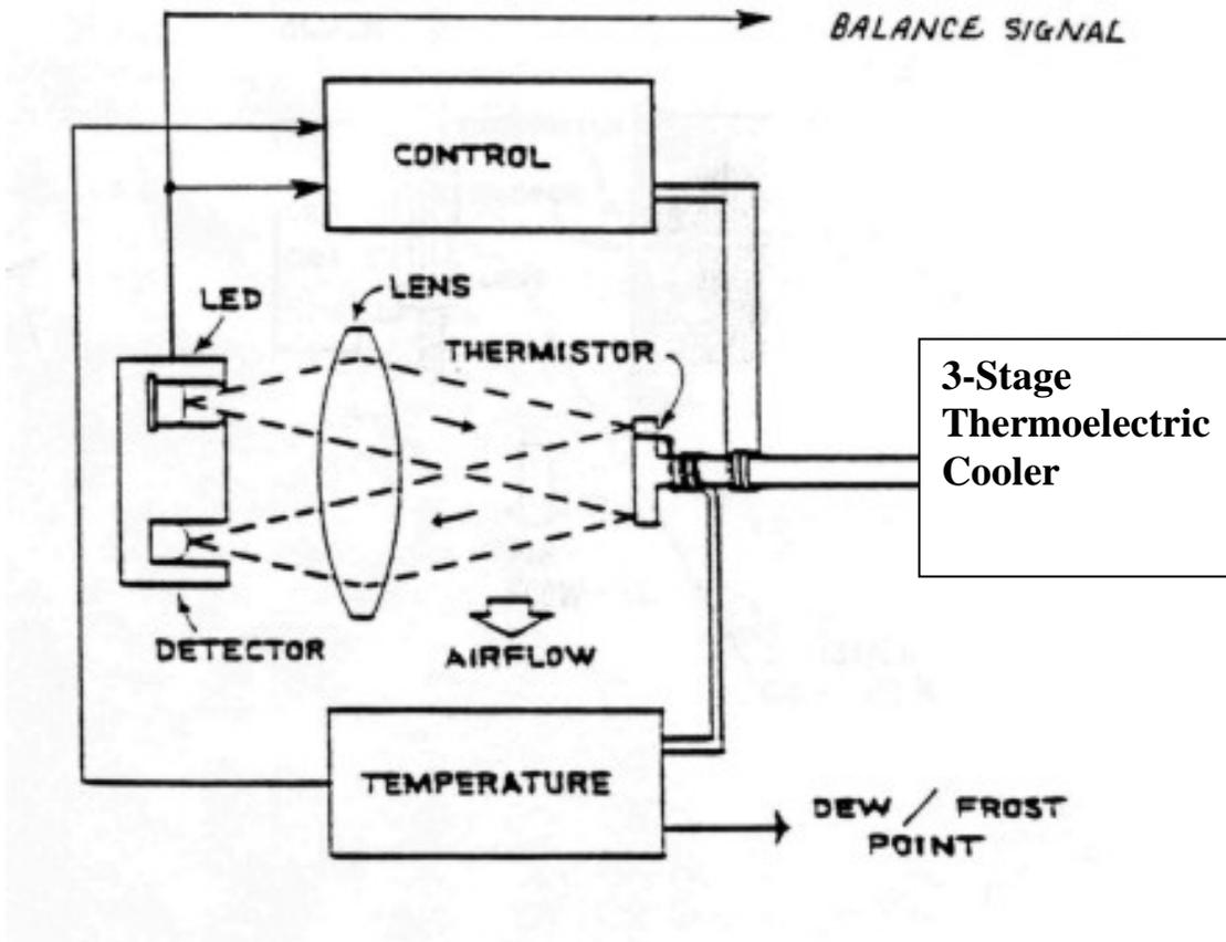
Fig. 3. Block diagram, CR-5 chilled mirror hygrometer
