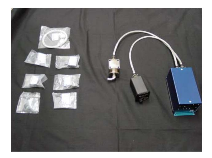
Figure 17. 1011C Hygrometer Complete
