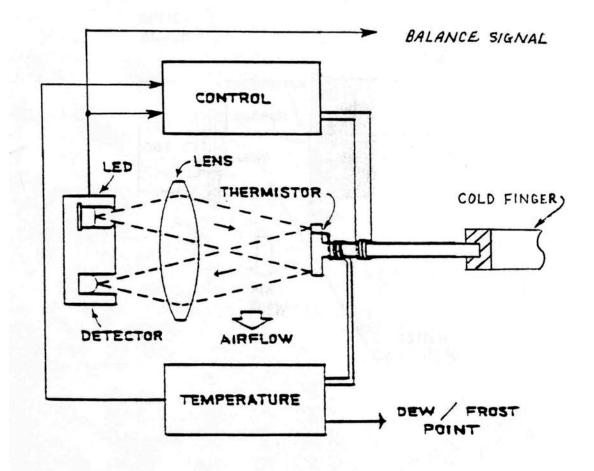
Fig. 3. Block diagram, CR-2 frost-point hygrometer
