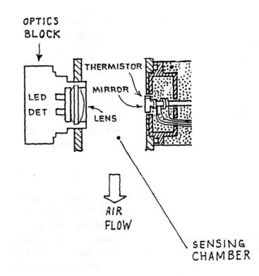
Fig. 4. Sensor assembly block diagram
