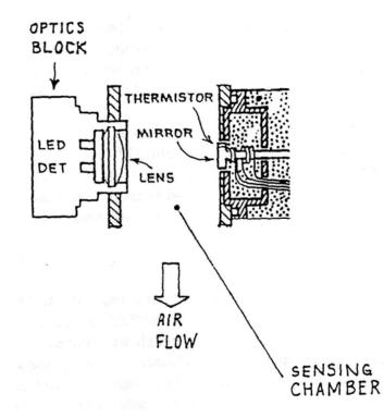
Fig. 4. Sensor assembly block diagram
