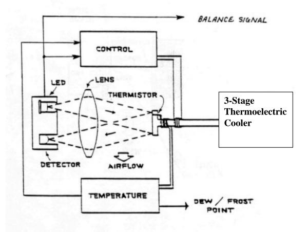
Fig. 3. Block diagram, CR-5 chilled mirror hygrometer
